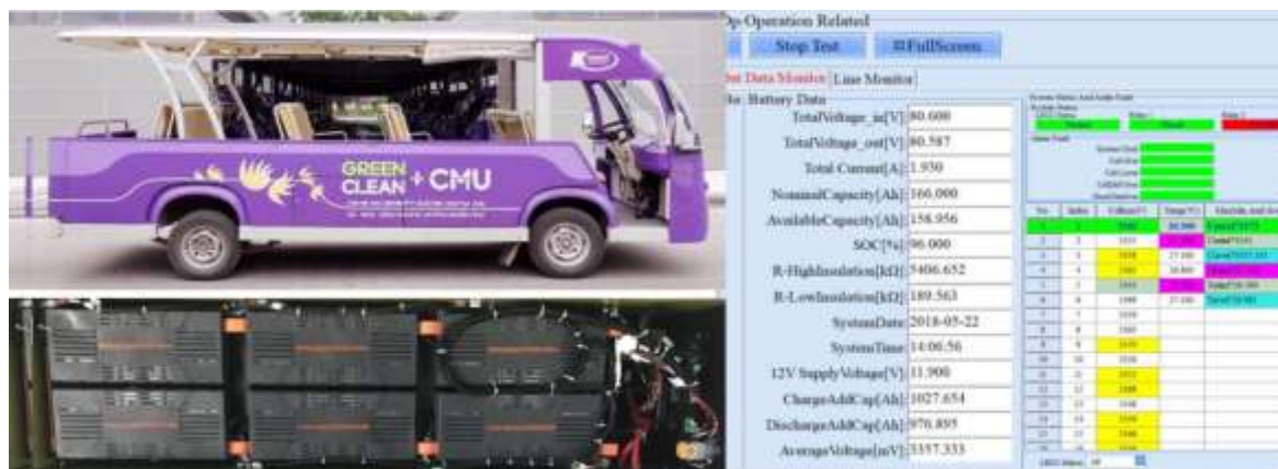
Figure 6. Electric bus and battery system
